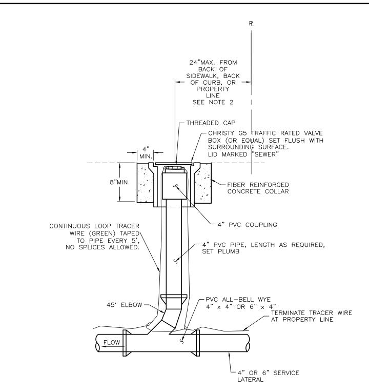
NOTE: ALL JOINTS AND CONNECTIONS SHALL BE WATERTIGHT.
