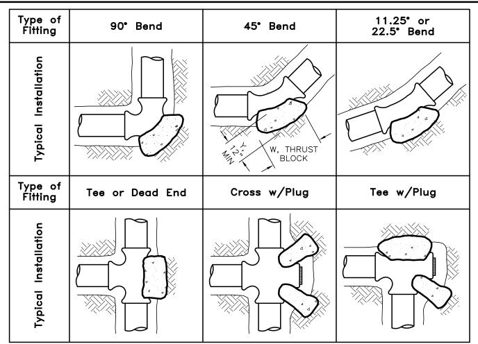
Minimum Thrust Block Bearing Area — Square Feet (Y x W)
